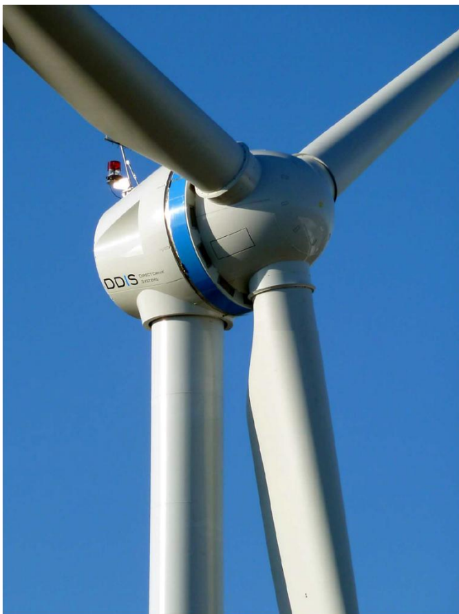
Fig. 1: Axial flux machine as generator integrated in a wind turbine.
