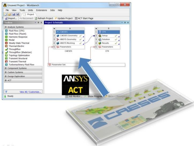
Fig. 2: ACT interface for integration of CAESES into the ANSYS Workbench platform.
