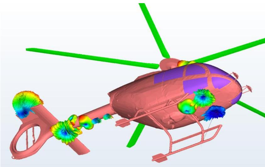
Fig. 2: Installed radiation pattern of the different antennas on the SH09 helicopter.
