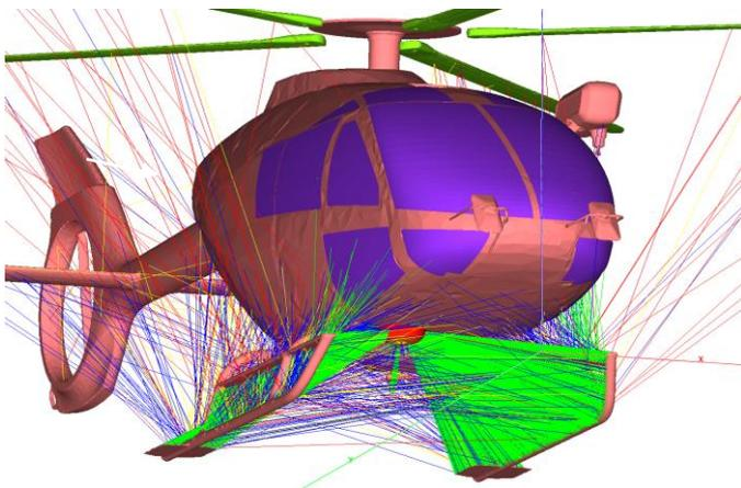
Fig. 3: Visualization of the shooting and bouncing rays for one specific VHF antenna (only electromagnetic rays, which bounce on the helicopter surface are shown).
